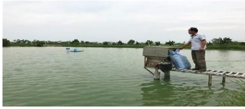
Figure 1. Fixed, single-speed fish feeder using a 220AC power source
